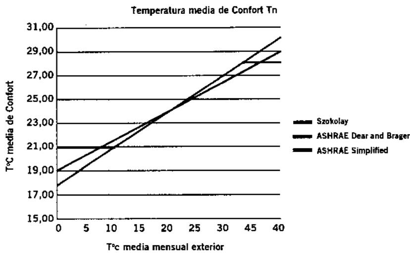
↑ Figura 16.21 Temperatura de confort neutral T<sub>n</sub>.
